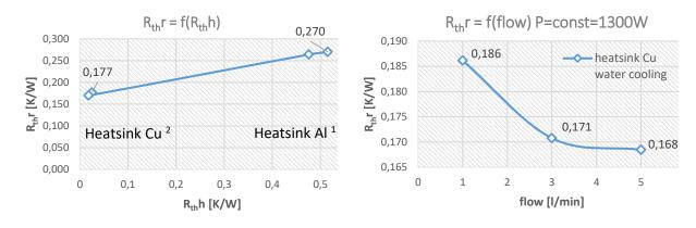
$R_{th}r$  – Thermal resistance of the RTS-02 resistor  $R_{th}r$  – Thermal resistance of the beatrink
