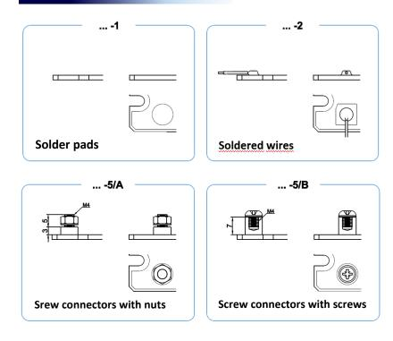
The recommended tightening torque for **5/A** and **5/B** connections is **1.2 Nm**
