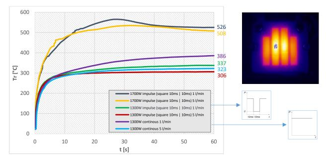
Tr – Temperature on resistor surface, Heatsink Cu<sup>2</sup> (water 21 °C), AAB TG4 thermal grease, 1,6 Nm mounting screws
