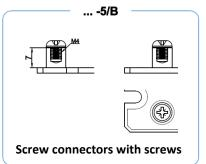
The recommended tightening torque for **5/A** and **5/B** connections is **1.2 Nm**
